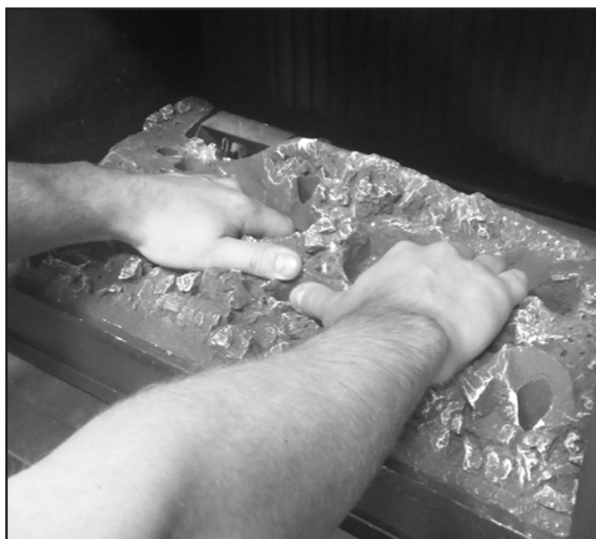
Figure 14. Burner Removal - Correct Hand Placement
